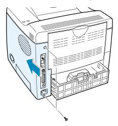
8 If you purchase the network interface card supporting the wireless LAN interface, insert the antenna counterclockwise, as shown.
